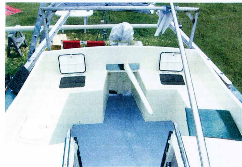
Topsides are constructed from ply covered with glassfibre cloth and resin
