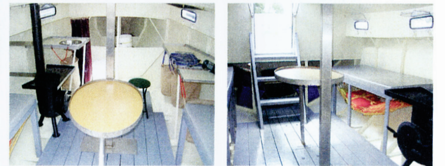
Functional down below. Note woodburning stove and stainless steel compression post
